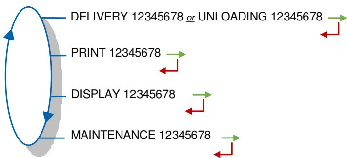
In USER mode, the AIRTRONIQUE displays a blinking figure which is the latest delivered quantity. On the prompter, you can see the name of the menu and the 8-char totaliser.
